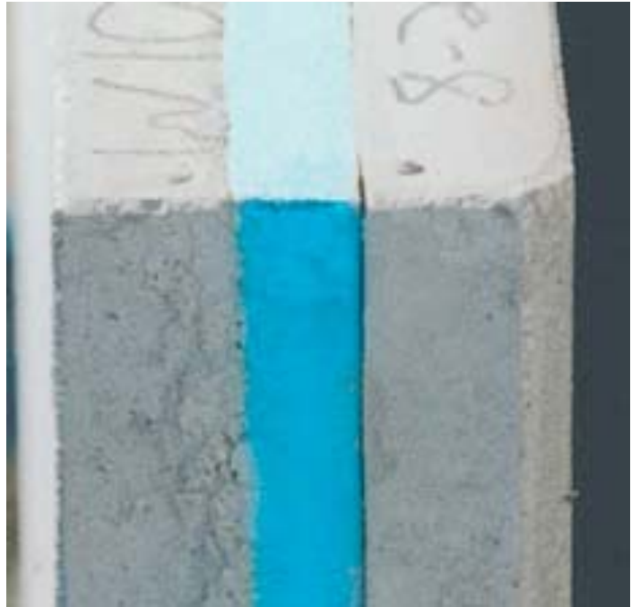
The Zero Energy Home's concrete walls feature both a high insulation value (as high as R-31) and insulated thermal mass exposed to the interior to dampen diurnal temperature swings
