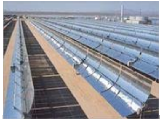
Parabolic Trough Concentrated solar power (high temperature solar thermal collector); source: Wikipedia.org : Solar Thermal Power
