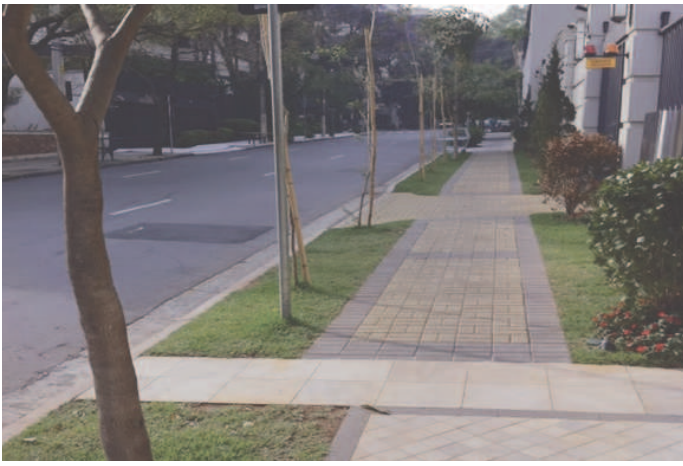
▲ Figure 157: Design error — the specification and detailing of too many special paving materials (photo: google images).
