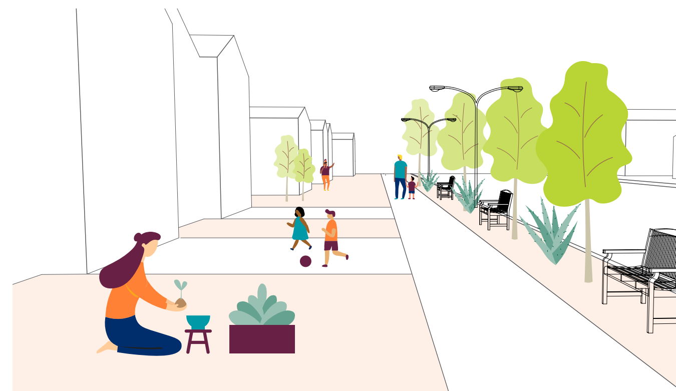
■ Conceptual illustration of a local street sidewalk, showing clear path of travel and an amenity zone between the sidewalk and the road, including trees, benches, and utilities.
