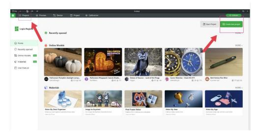
Makers can import models from the *Create New Project* button, located at the top right of the screen, which will open the *Prepare* section, or open the *Prepare* section itself. The *Prepare* section opens the build viewer with the printer specifications on the left-hand side. The import model button is located on the far left of the toolbar.
