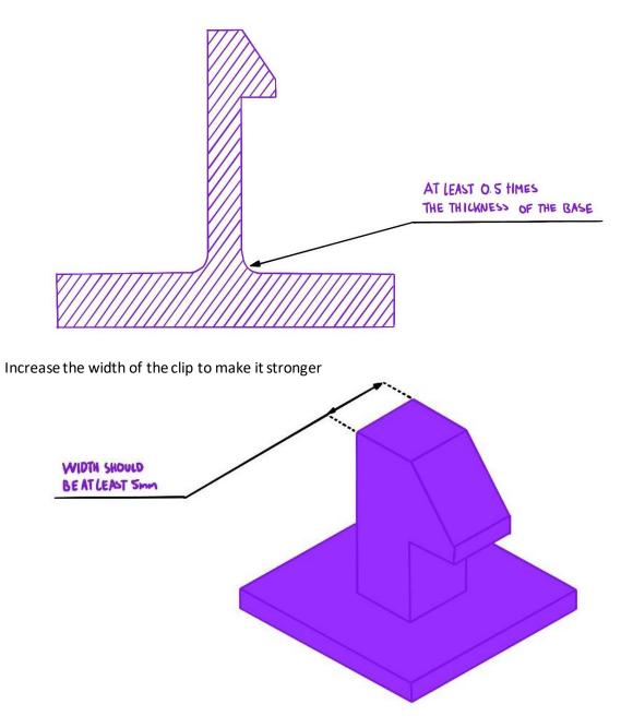
• Consider the build direction. Avoid designing snap-fit cantilevers that are built up vertically because they are inherently weaker.
