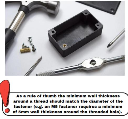
If the wall thickness is too low, the parts can distort or fracture due to the added stress.
