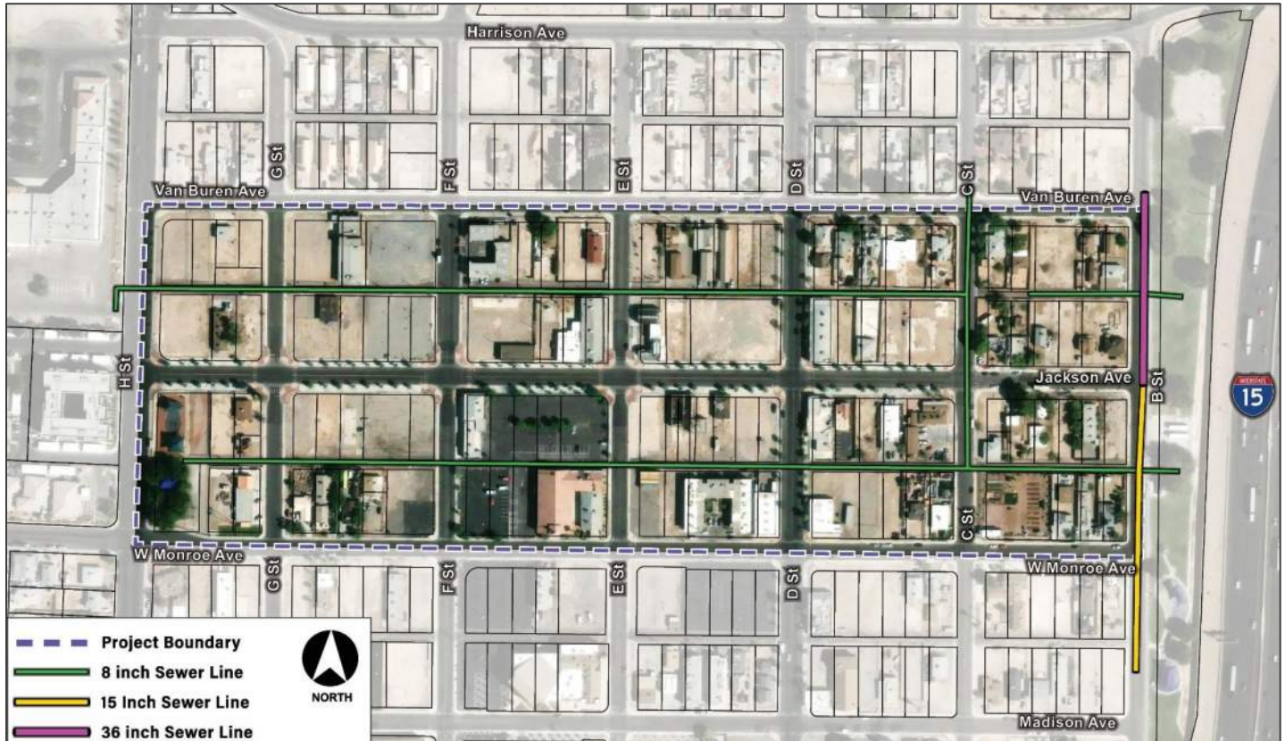
Figure 14: Existing Sewer Lines Map
