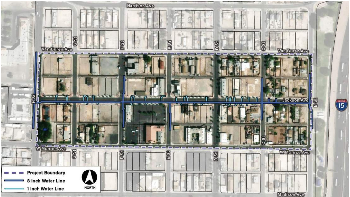
Figure 15: Existing Water Lines Map
