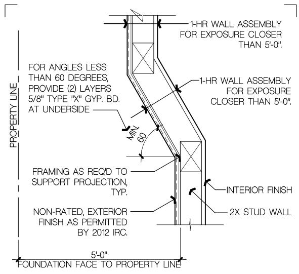
THE PROJECTION CONDITION DEPICTED HERE APPLIES TO MEDIA NICHES, BAY WINDOWS, AND OTHER SIMILAR PROJECTIONS THAT DO NOT CONTAIN OCCUPIABLE FLOOR SPACE. FOR PROJECTIONS OR CANTILEVERS SUPPORTING FLOOR SPACE ABOVE, SEE 1-HR PROJECTION DETAIL P4.
