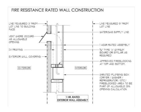
TABLE R302.1(1) - WALLS REQUIRED TO BE FIRE RESISTANCE RATED AND MEASURED A MINIMUM 3'-0" TO BUILDING FACE FROM PROPERTY LINE ARE PERMITTED 25% MAXIMUM OF WALL AREA AS UNPROTECTED OPEN.
