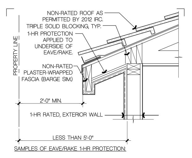
1. EXT. FINISH O/ (2) LAYERS 5/8" TYPE "X' GYP. BD. APPLIED TO UNDERSIDE OF EAVE FRAMING SPACED 24" MAX.
