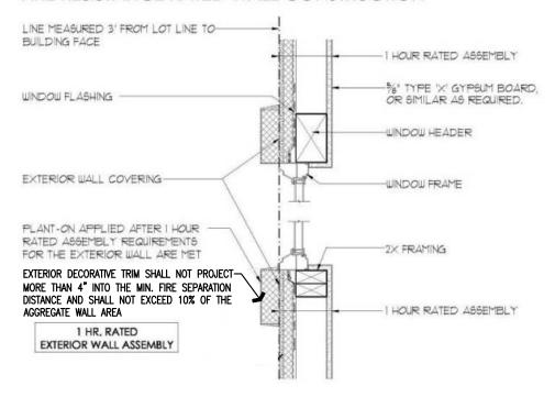
TABLE R302.1(1) - WALLS REQUIRED TO BE FIRE RESISTANCE RATED AND MEASURED A MINIMUM 3'-0" TO BUILDING FACE FROM PROPERTY LINE ARE PERMITTED 25% MAXIMUM OF WALL AREA AS UNPROTECTED OPEN.
