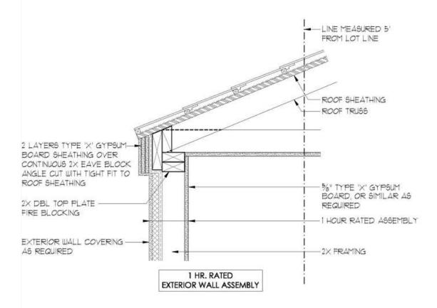
IF 3" MINIMUM SOLID MATERIAL IS PROVIDED AT THE EAVE AND PROTECTED BY 2 LAYERS 5/8" TYPE 'X' GYPSUM BOARD SHEATHING, THE INTERIOR SURFACE OF THE FIRE-RATED WALL ASSEMBLY IS NOT REQUIRED TO EXTEND TO THE ROOF SHEATHING, OTHERWISE IT SHALL EXTEND TO THE UNDERSIDE OF THE ROOF SHEATHING.
