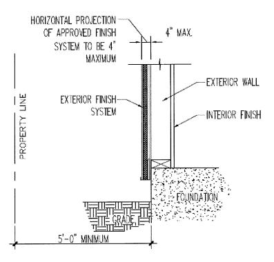
NOTE: INTERICR AND EXTERIOR WALL FINISH SHALL CONTINUE TO FULL HEIGHT OF WALL.
